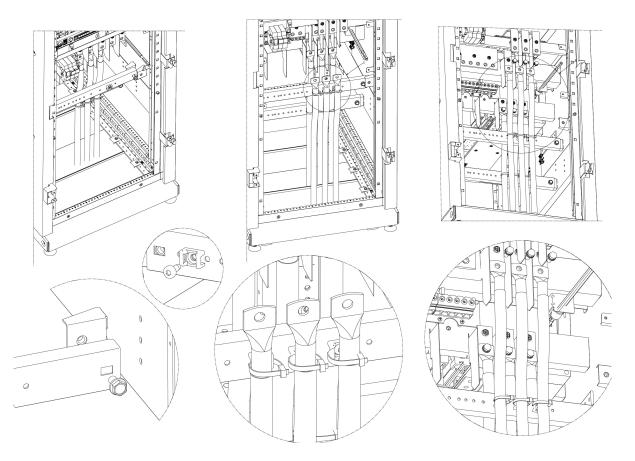
KEOR MOD 250 – fixing of the bar and fastening of the neutral and bypass cables
