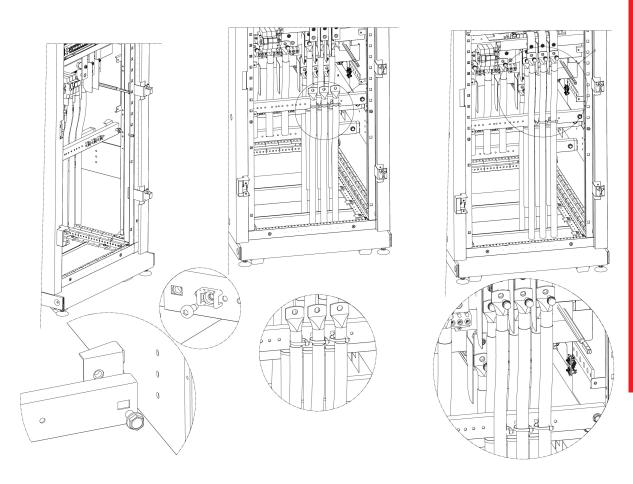
KEOR MOD 250 – fixing of the bar and fastening of the input cables
