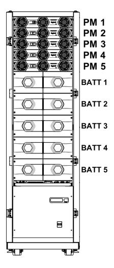
Starting from the top of the cabinet, unscrew the four screws that fix the slot cover where the battery drawers must be installed and save them.
