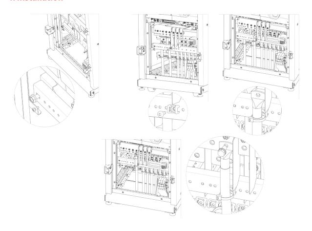
KEOR MOD 125 – fixing of the bar and fastening of the neutral and bypass cables
