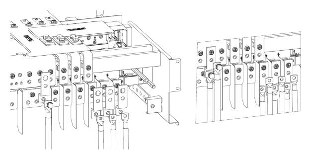
KEOR MOD 125 – neutral and output cables installation with accessory for double cable
