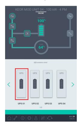
3. Choose the PM to replace by tapping on it or scrolling it with the ARROWS UP and DOWN icons. Then, tap on the SWITCH icon and confirm to turn off the module once the pop-up appears.
