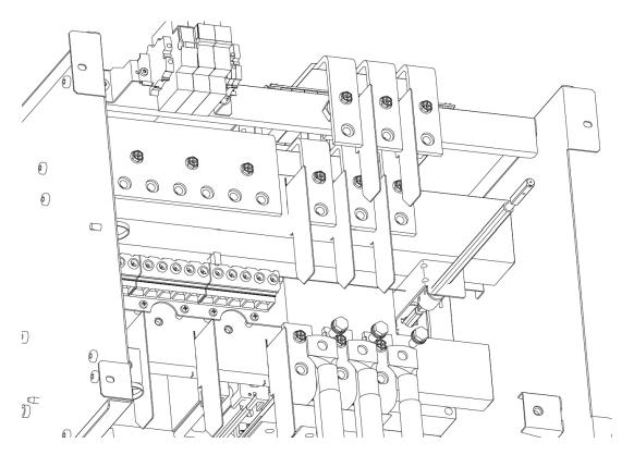
**KEOR MOD 250 – output cables installation**
