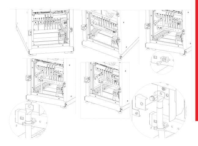
KEOR MOD 125 – fixing of the bar and fastening of the battery, input and output cables
