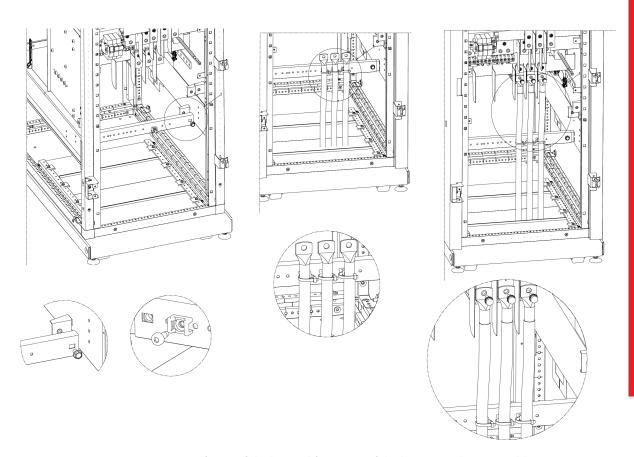
KEOR MOD 250 – fixing of the bar and fastening of the battery and output cables
