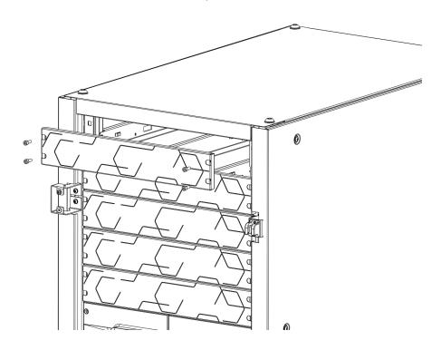
Insert the power module in the free slot, making sure that its switch in the front is open.
