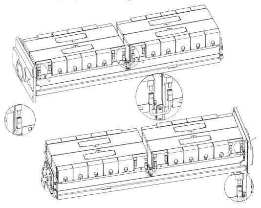
Insert the remaining terminal covers on the batteries.
