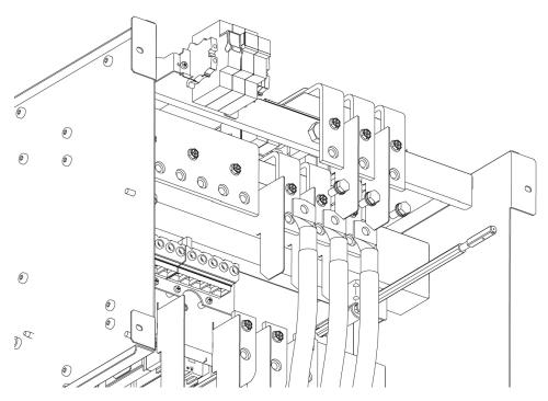
**KEOR MOD 250 – bypass cables installation**
