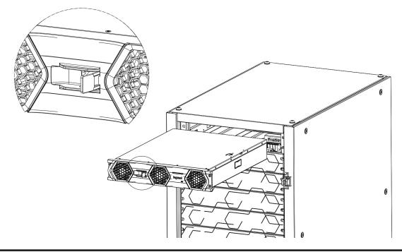
Make sure that the power module is abut and then close its front switch. Fix the module to the cabinet with the four screws that were previously saved.
