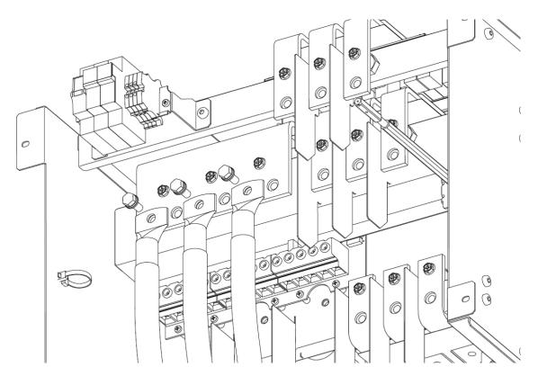
**KEOR MOD 250 – neutral cables installation**
