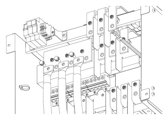
**KEOR MOD 250 - neutral cables installation**
