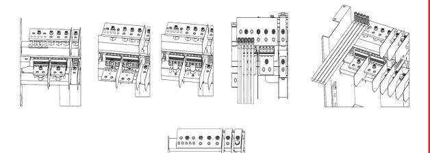
KEOR MOD 125 – batteries cables installation with independent strings of batteries
