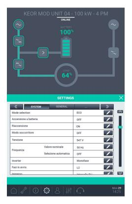
7. Set the correct number of KB (Battery Kits) installed in the tab "System" **INDICATION**
