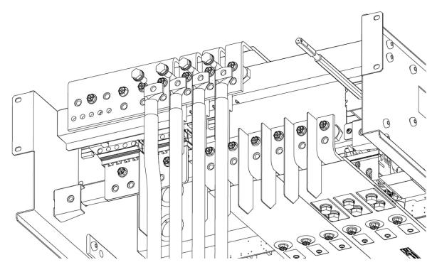
KEOR MOD 125 - neutral and bypass cables installation
