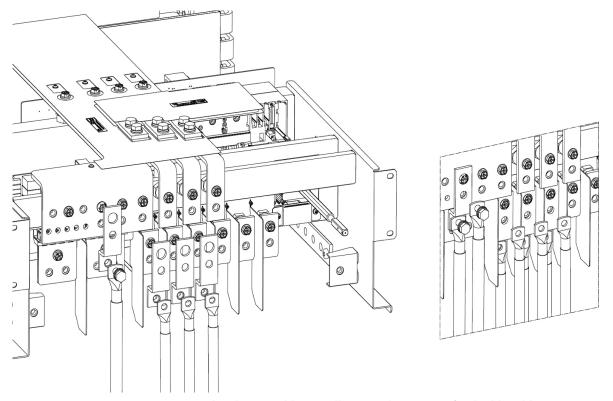
KEOR MOD 125 - neutral and input cables installation with accessory for double cable
