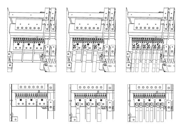
KEOR MOD 250 - batteries cables installation with strings of batteries in common
