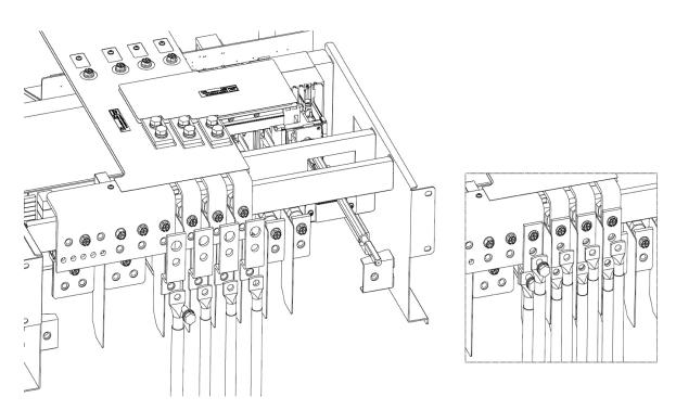
KEOR MOD 125 – neutral and bypass cables installation with accessory for double cable
