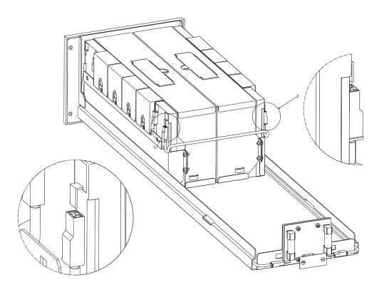
Once the connection is done, insert the terminal covers on the two batteries and push the blocks at the bottom of the drawer.
