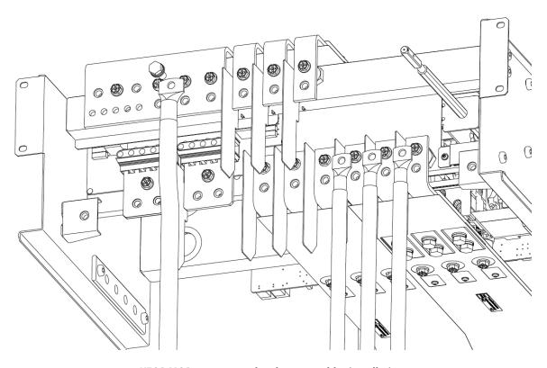
KEOR MOD 125 - neutral and output cables installation
