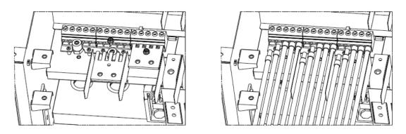
KEOR MOD 250 – batteries cables installation with independent strings of batteries
