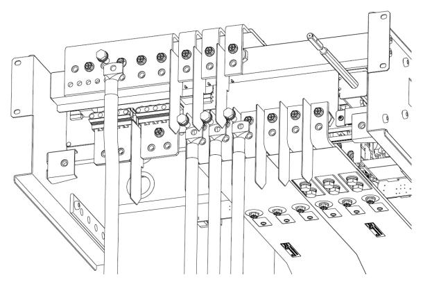
**KEOR MOD 125 – neutral and input cables installation**
